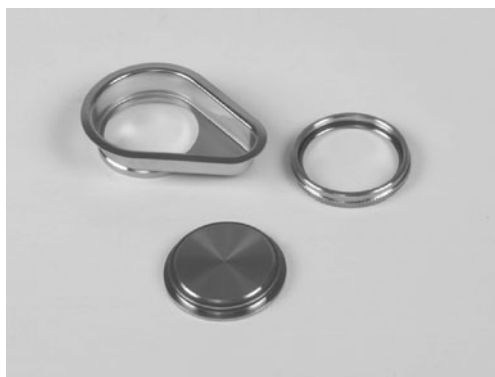
Fig. 2. Modified NGI dissolution cup (reproduced with permission from Copley Scientific Limited UK)
